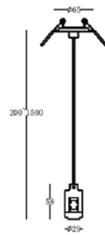
Pendant- Recessed flexible fastening+ Electric Cable(max 1200mm)
